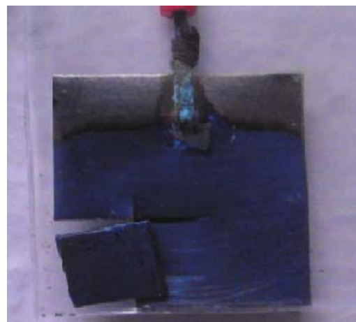
Fig.3 Cooper wire of the sample of TiO 2 after anodizing covered with light blue reactant.
